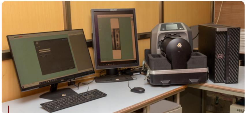
Artificial Intelligence (AI) enabled weld inspection tool with computerized radiography (AI-RT)
