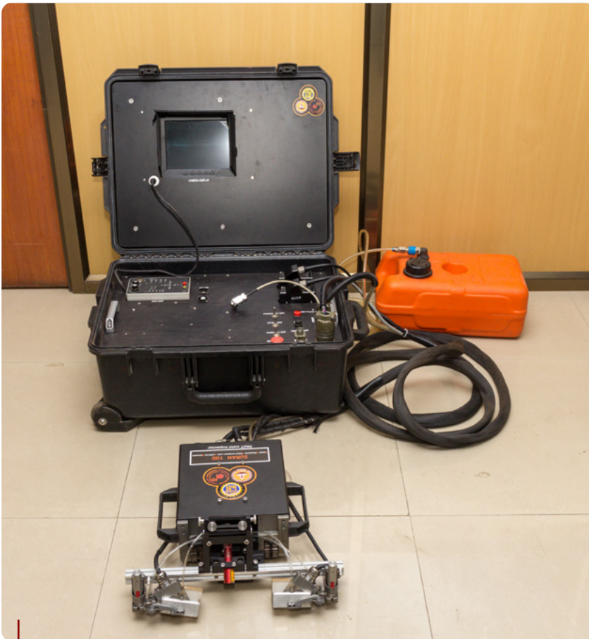
Artificial Intelligence (AI) enabled weld inspection tool using advanced phased array technique to replace manual radiography (AI-UT)
