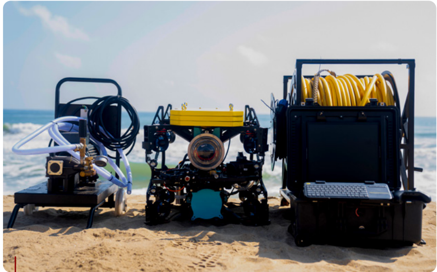
Artificial Intelligence (AI) enabled remotely operated vehicle (AI-ROV) for under water inspections
